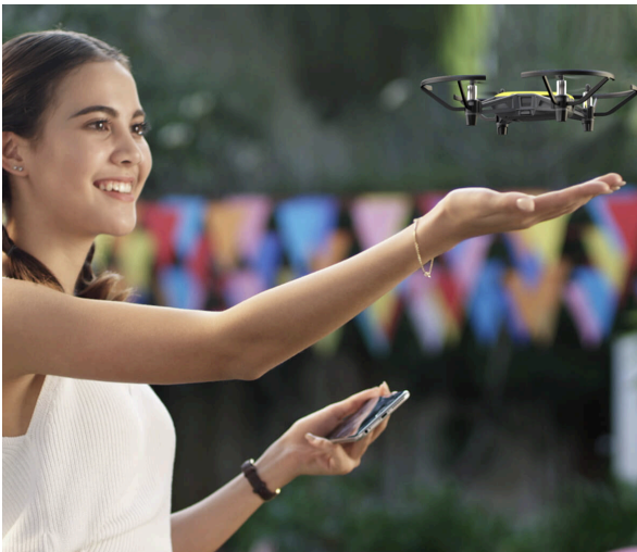
DJI Tello Drone auto landing to the nearest surface, in this case the user's hand, due to not receiving any input
